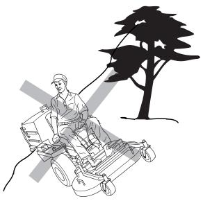
Figure 4-8 Improper Operation on a Slope
